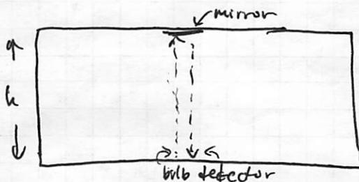
Consider another car at rest. A flash bulb at the bottom flashes, reflects off a mirror, and is detected. Clock at this location reads a time,  $\Delta t = 2h/c$
