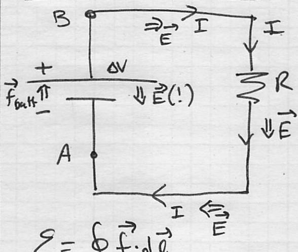
In this simple circuit, the Battery drives a current  $I$  through the wires / resistor  $R$ .
