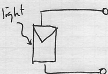
A photovoltaic device that converts light (photons) into electrical energy
