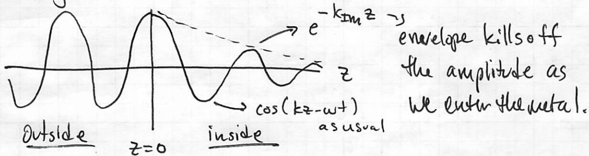
The wave dies out ( $1/e$  factor) in a distance,
