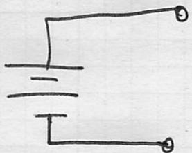
A battery that through chemical reactions creates a potential difference
