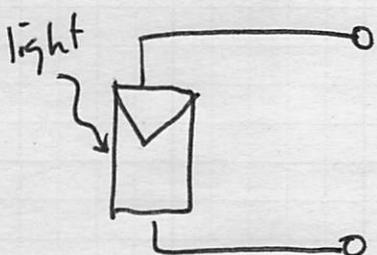
A photovoltaic device that converts light (photons) into electrical energy
