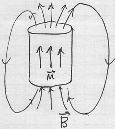
So it's a permanent magnet, which looks like a finite solenoid (inside & outside) even though there is no 'wire' with current wrapped around it.
