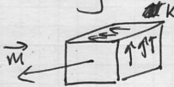
a little surface current  $K$  running around these 4 surfaces could give rise to  $\vec{m}$ .
