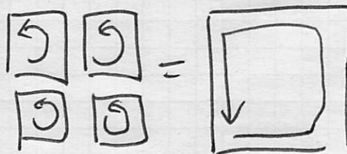
So a solid material with uniform tiny atomic currents can be modeled as simply having a macroscopic current running all around the surface of the material.
