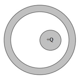
Consider how the charge distribution would change if the inner conductor is shifted off-center, but still has +Q on it, and the outer conductor remains electrically neutral. Draw the new charge distribution (little + and – signs) and be precise about how you know.
