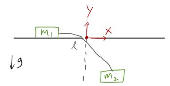
Two masses  $m_1$  and  $m_2$  are connected by a massless rope of length  $\ell$ . As pictured, one of them rests on a frictionless table, while the other is dangling over the edge. We'll treat this as a **two-dimensional** system, starting with Cartesian coordinates (x, y) as depicted. Note that in particular, this means that **block 2** is free to swing back and forth!
