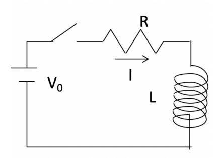
The switch is closed at t = 0. Which graph best shows I(t) through the resistor?
