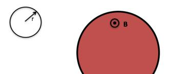
The current in an infinite solenoid with uniform magnetic field  ${\bf B}$  inside is increasing so that the magnitude B in increasing with time as  $B=B_0+kt$ . A small circular loop of radius r is placed outside the solenoid as shown.
