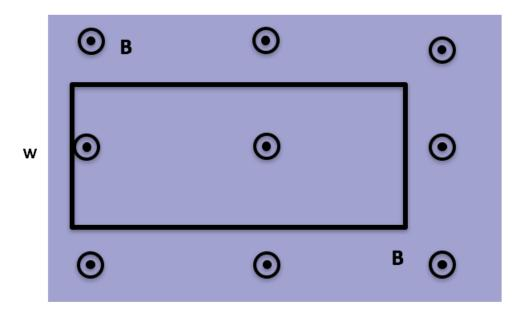
A rectangular metal loop is moving thru a region of constant uniform magnetic field  ${\bf B}$ , out of page, with constant speed v, as shown. Is there a non-zero emf around the loop?
