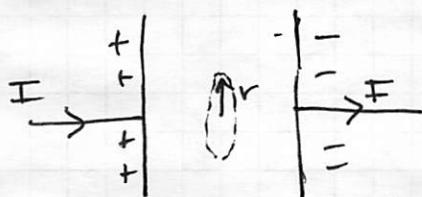
we choose a circular loop that is plane parallel to the plates.  $d\vec{A} = \hat{\phi} d\phi dS \hat{z}$
