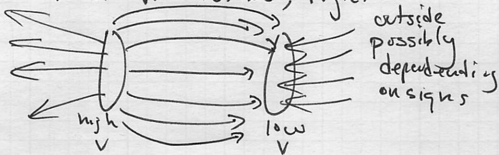
The cylindrical conductor charges flies. the current can't leave the conductor for free space, hence  $\vec{J}$  is confined to the conductor, thus  $\vec{E} = \vec{J}/\sigma$  is as well.\*
