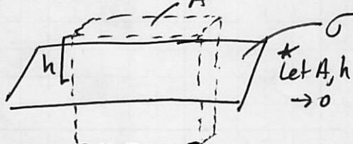
A small Gaussian "pill box" around a sheet of charge with  $\sigma$  surface charge.
