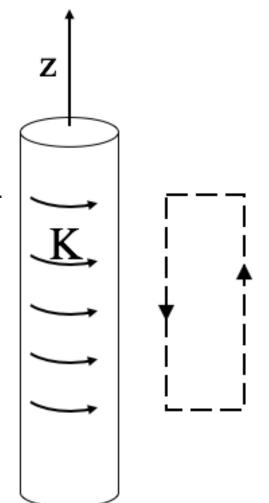
An infinite solenoid with surface current density K is oriented along the z-axis. Apply Ampere's Law to the rectangular imaginary loop in the yz plane shown. We can safely assume that  $B(s \rightarrow \infty) = 0$ . What does this tell you about the B-field outside the solenoid?
