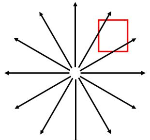
This picture represents the field lines of a single positive point charge.
