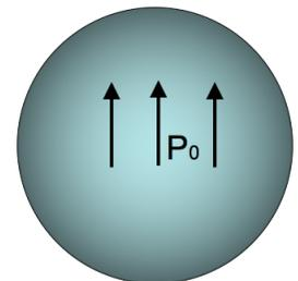
A dielectric sphere is uniformly polarized,
